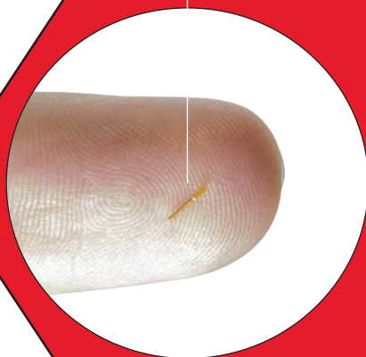
RF MICRO-RELAY A DC-8 GHz switch that can 'hot' switch RF signals
